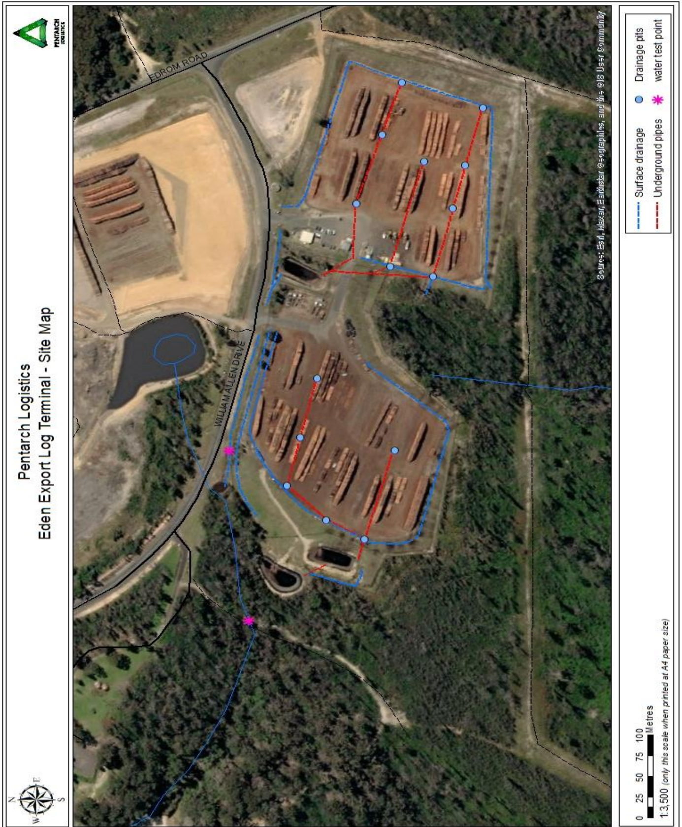
Figure 2: Export Log Yard Water Management Components
